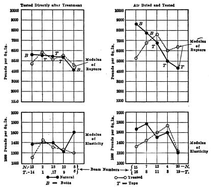
Fig. 18.—Effect of preservative treatment on the strength and stiffness of longleaf-pine stringers treated partially air dry.
